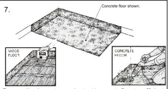
Remove the shower tray and cut out / excavate floor to sufficient depth to accept the shower trap (approximately 110mm width and 150mm depth). Extend the cut out / excavated area to the wall.
