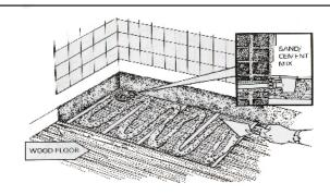
Before bedding the tray into position, use a weak sand and cement mix to fill the void underneath the shower tray. Carefully fill the area around the shower trap.
