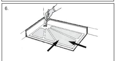
Fit tray in recess, push back into the wall cut-out. Mark the position of the trap.
