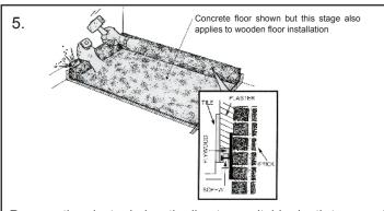
Remove the plaster below the line to a suitable depth to accept the tiling lip. Use plywood to pack out if necessary.
