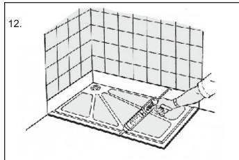
Finally, fill any gaps at the edges of the shower tray with silicone sealant.
