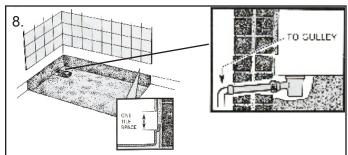
Cut through the wall to accommodate the waste pipe if required. Fit shower trap to waste pipe. **DO NOT FIX IN PLACE.** Check the trap can be aligned with the hole in the tray to enable fitting of trap 'screw top'. Measure one tile space above the tiling lip position. Tile walls above, leaving one row untiled as shown.
