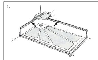
Place the shower tray in the corner to which it will be finally positioned. Mark lines along the two walls above the upper edge of the tiling lip. Mark the outline of the tray onto the floor.
