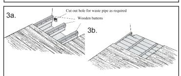
Wood Floors ONLY: Cut and remove floorboards. Trim any obstructions such as floor joists to ensure the tray sits in the space. Screw battens to each joist (3a), Use 20mm thick plywood, or similar, to form a platform between the joists (3b).
