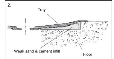
Wooden & Solid Floors: An area of approximately 40mm in depth must be removed to accept the shower tray. Solid Floors Only: Concrete / Screed should be removed to a depth of 40mm, as shown by dimension 'A'.
